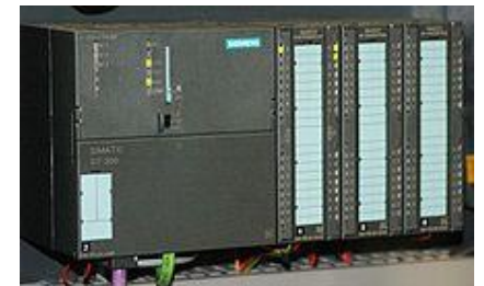
Siemens Simatic S7-300 PLC CPU with three I/O modules attached
